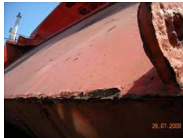
Top portion of door structure wasted and holed
